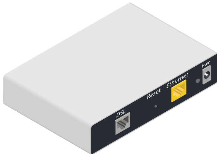
RJ-11 DSL (left) and RJ-45 LAN (right) ports on a DSL modem. (Image © 123RF.com.)
