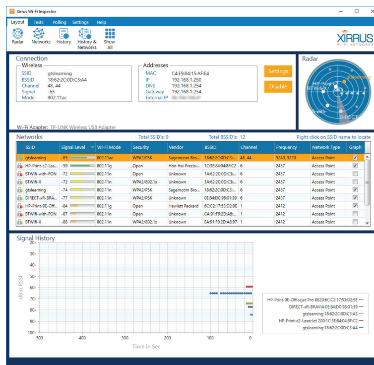
Surveying Wi-Fi networks using Xirrus Wi-Fi Inspector (xirrus.com)—Note the presence of print devices configured with open authentication (no security) and a smart TV appliance (requiring authentication). (Screenshot used with permission from Xirrus.)
