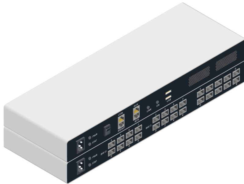
USB and RJ-45 type console ports plus AUX and other management interfaces on a router. (Image © 123RF.com.)
