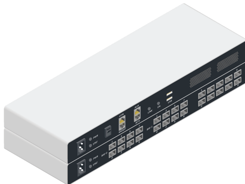
An advanced services router. This type of device provides network edge connectivity over Carrier Ethernet networks. (Image © 123RF.com.)
